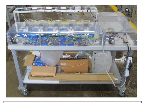
Bowmar's current 5-bay immersion tester. It is expected that only the cart/bench, (5) individual dunk tanks, fans, and fan mount(s) are to be re-used. All plexiglass covers and electronics to be removed and replaced with components appropriate for an industrial environment.
