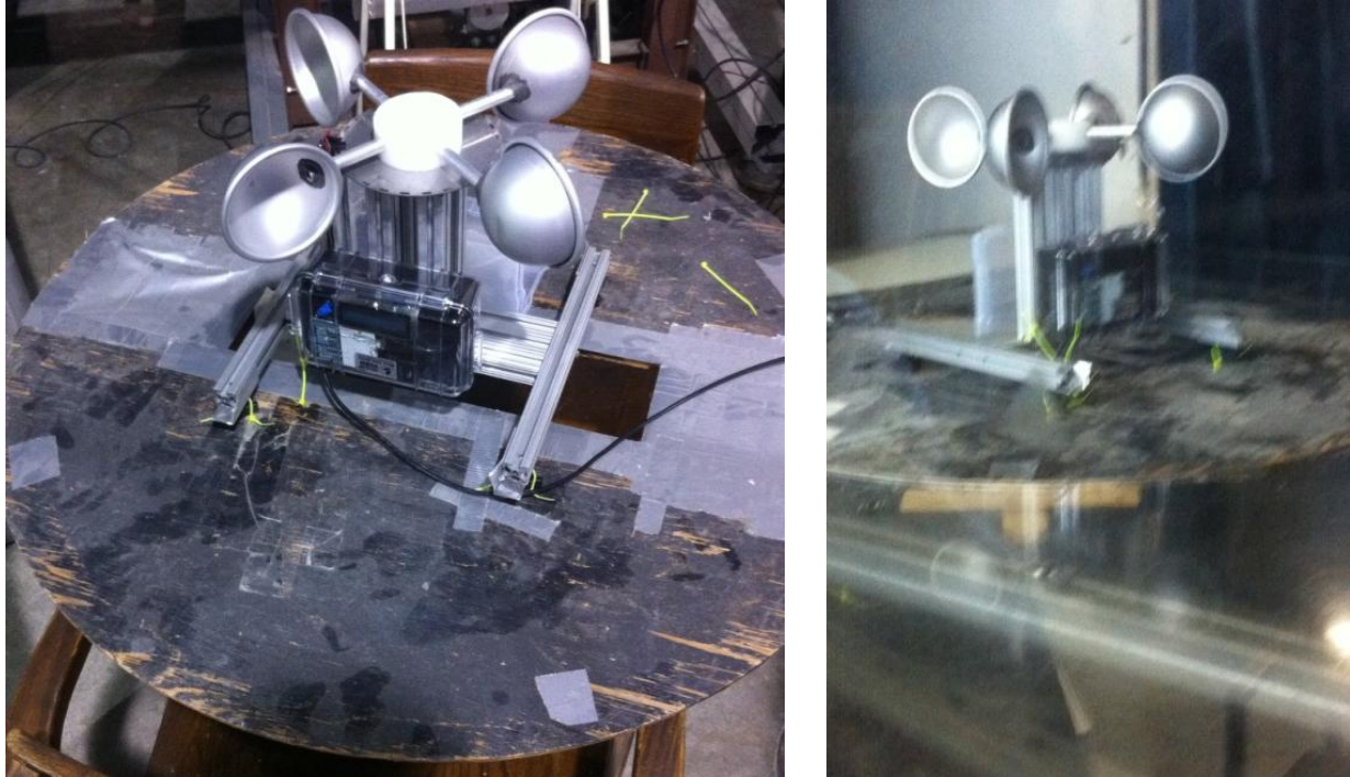
(Left) Figure 3.3-x: Zip Tying Down the Anemometer (Right) Figure 3.3-y: The Anemometer Placed in the Wind Tunnel
