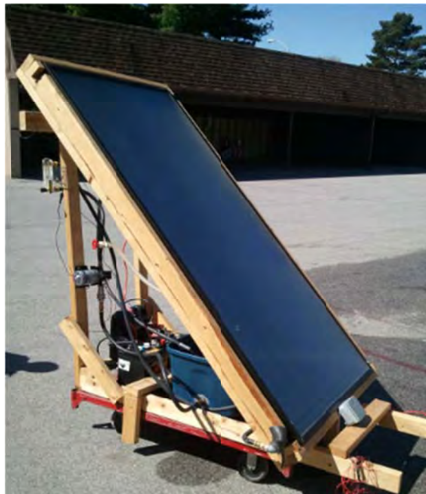
Figure 5.2: side view of the utilized solar collector
