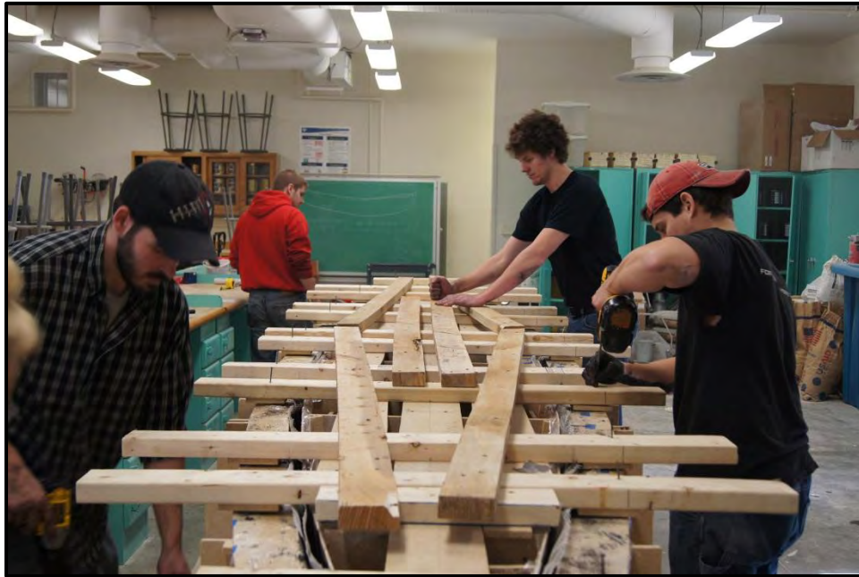
Figure 12: The interior mold being attached to the exterior mold.
