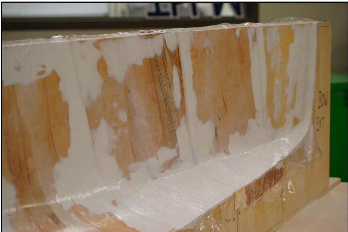
Figure 5: Thin layer of plastic applied to the exterior mold.
