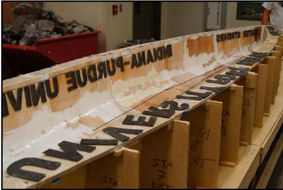
Figure 5: Vinyl inlays being attached to exterior wood mold to create school name and theme name in concrete canoe.
