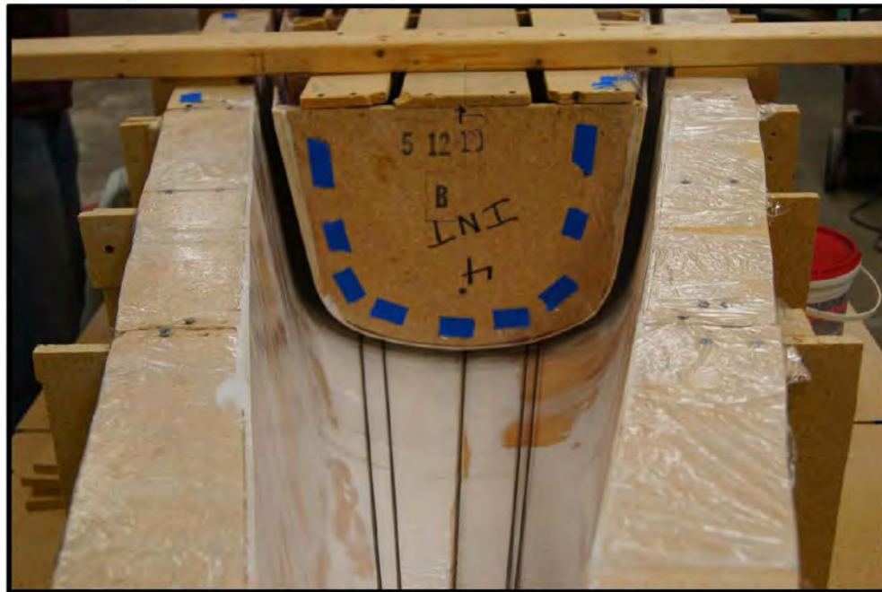
Figure 4: Interior Mold and Exterior mold configuration to obtain consistent 1" thickness.
