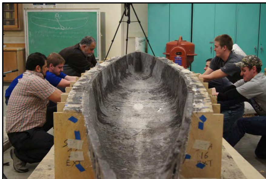
Figure 16: Removing the exterior mold from the canoe.
