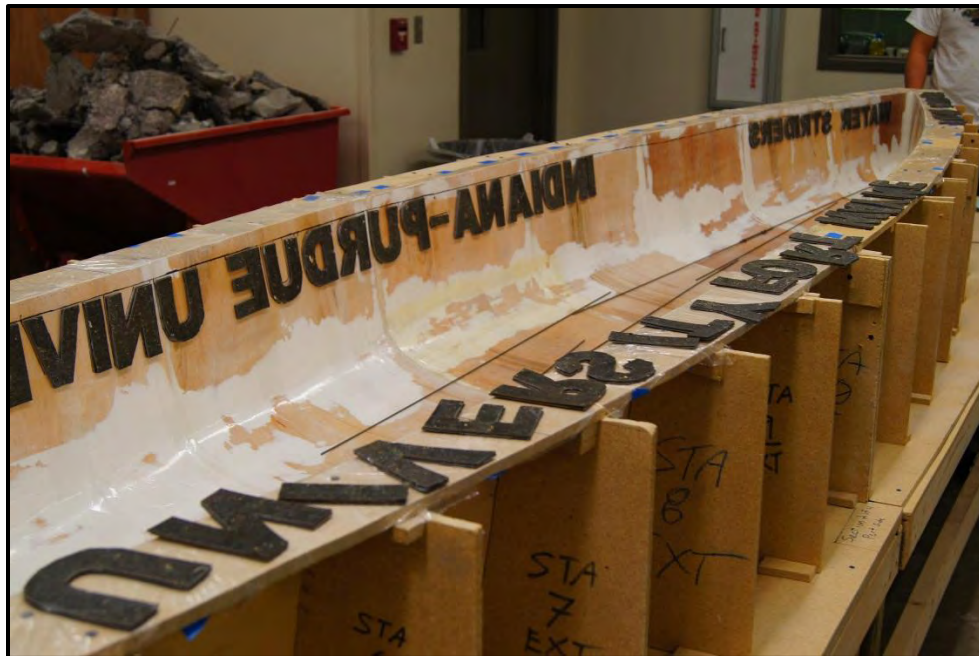
Figure 8: The vinyl inlays for the school name and canoe name being attached.
