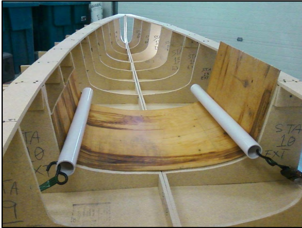
Figure 4: Applying the soaked plywood to the canoe skeleton.
