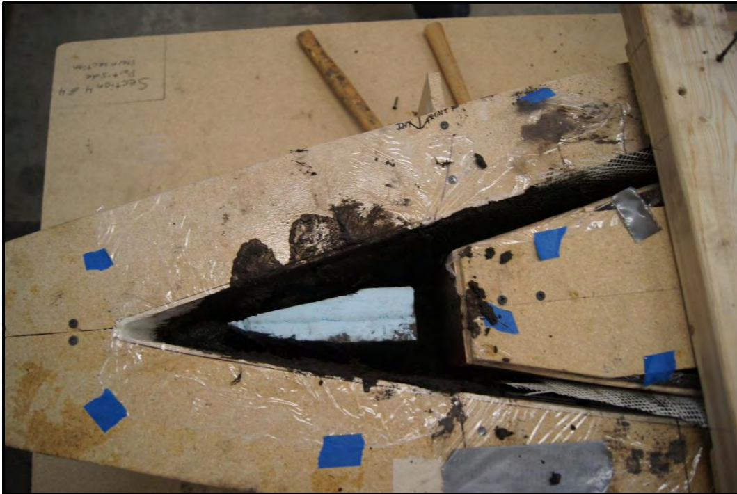
Figure 14: Rigid foam wedge being placed in the bow.
