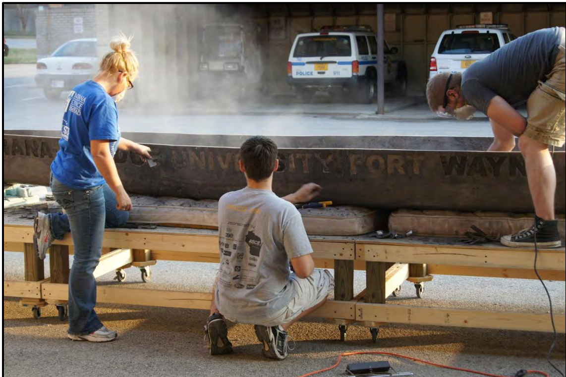
Figure 19: The design team starting to rough sand the canoe.
