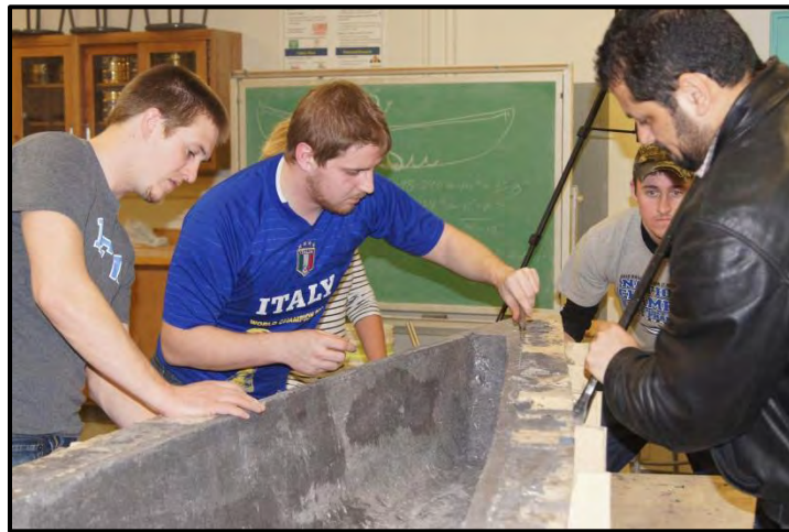
Figure 15: Starting to de-mold with crow bar.
