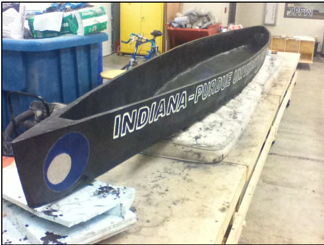
Figure 23: The final canoe product with two coats of the clear sealer applied.
