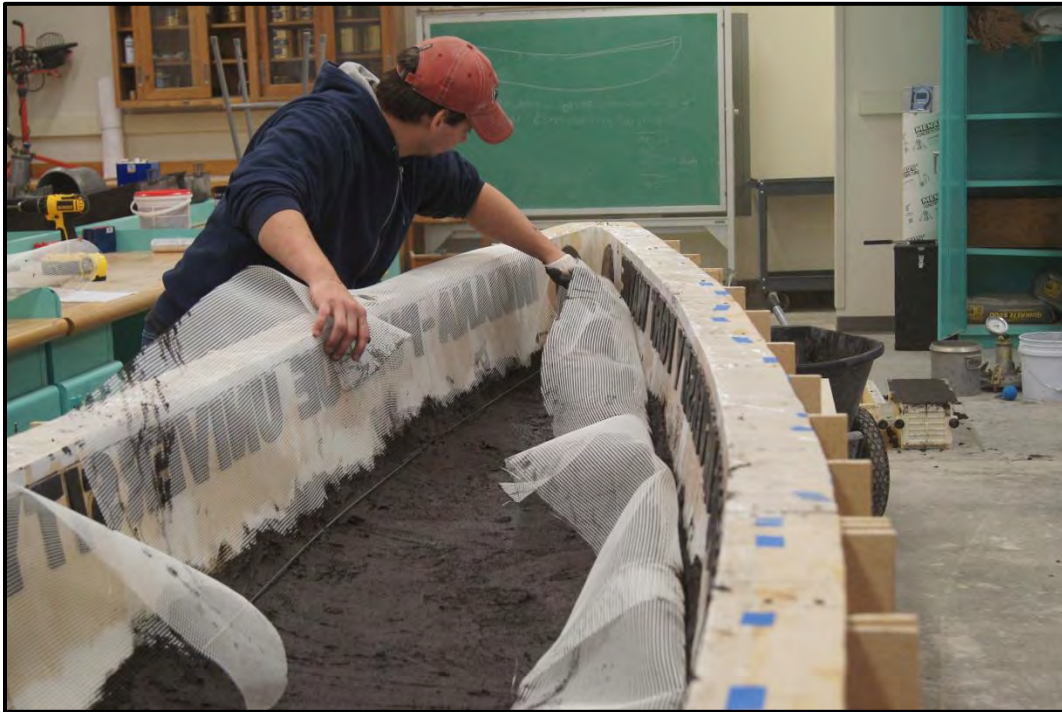
Figure 11: Reinforcing fiberglass mesh being added, along with steel bars.
