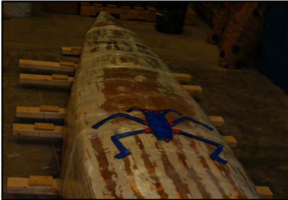
Figure 6: Water strider vinyl inlay attached to interior mold to create graphic on the interior section of the canoe.
