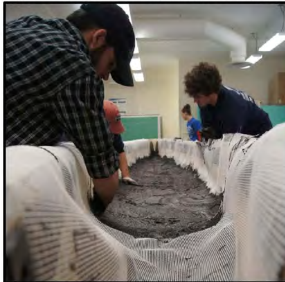
Figure 10: Placing the second layer of fiberglass grid reinforcement.
