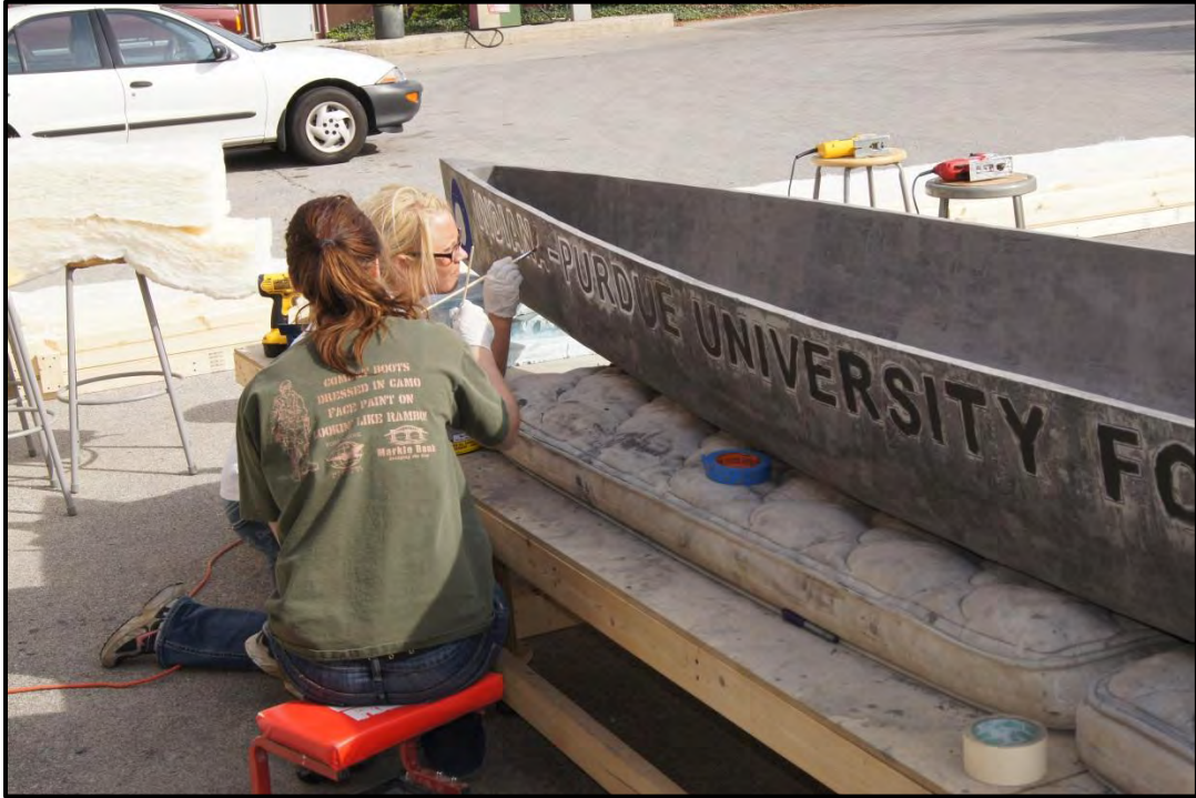
Figure 22: Applying the concrete paint to the lettering.
