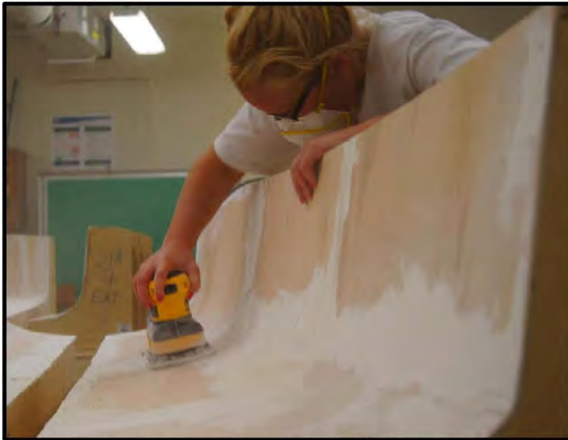
Figure 1: Sanding the exterior mold to give a smooth finish for the concrete canoe.
