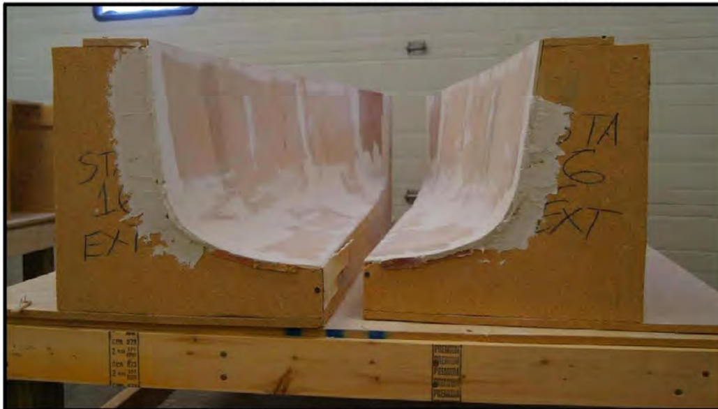
Figure 2: Displaying the ability to separate the mold for future changes in dimensions as well as ease in de-molding.
