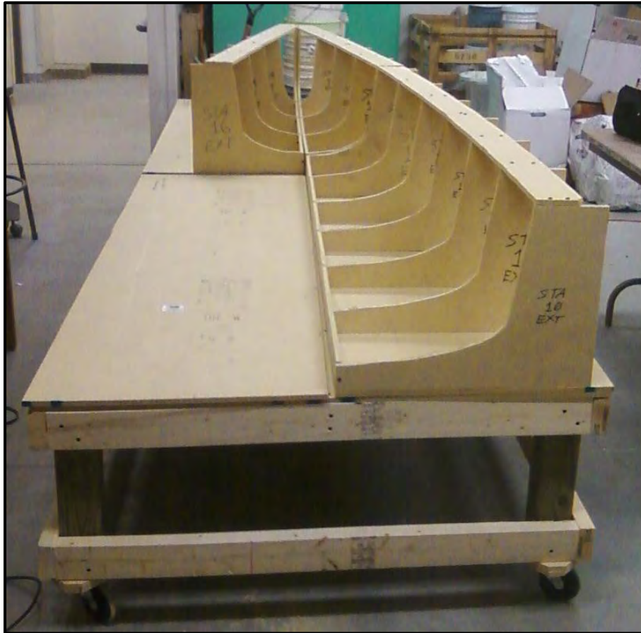
Figure 3: Skeleton of canoe being constructed on top of base.
