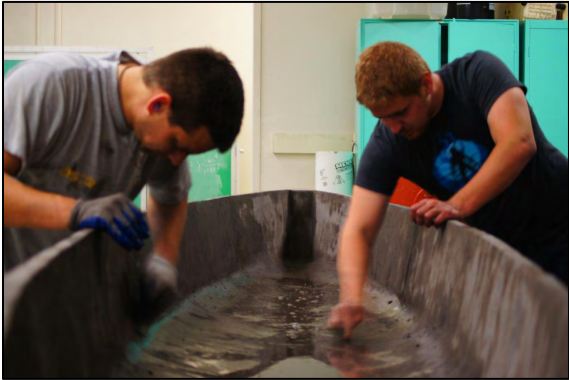
Figure 20: The design team wet-sanding the canoe.
