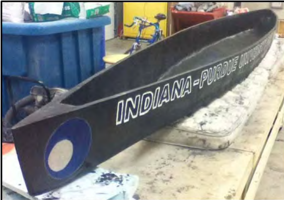
Figure 16: Finished canoe with two coats of sealer applied.
