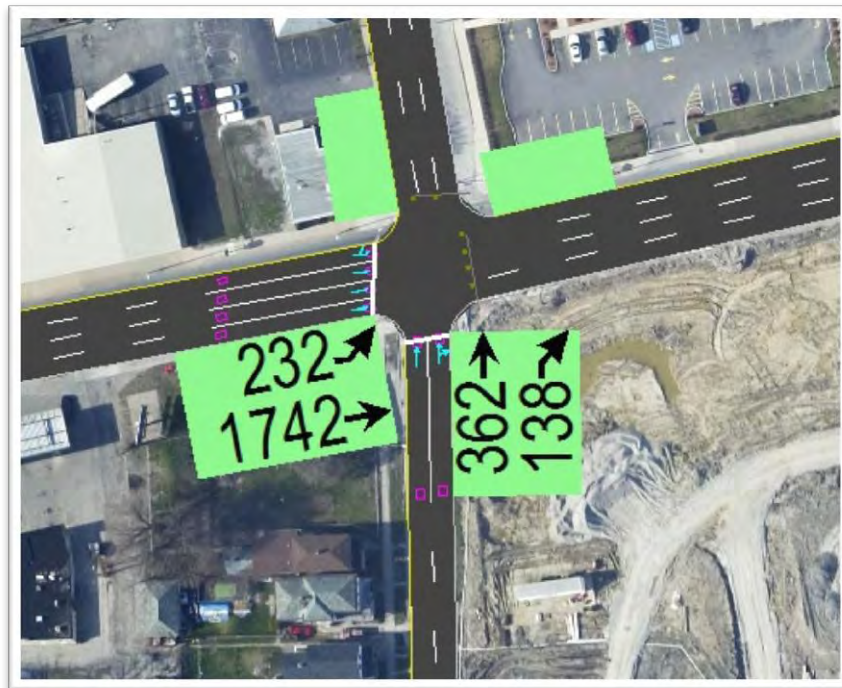
Figure 8 – Modeling with Synchro 7
